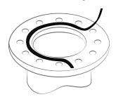
The other end of the sealing tape is placed over the skived end and any excess material is cut off at an angle, making sure the total thickness is approximately 120 % of the original sealant tape thickness.
