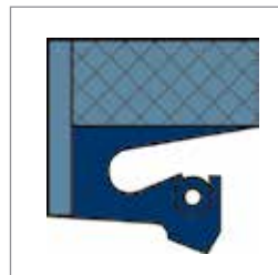
Model 154-P Universal Oil Seal 154-P incorporates radial lubrication grooves.
