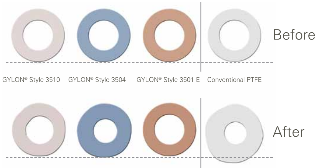
A comparison between GYLON® flat gaskets and un-filled PTFE after exposure to a load of 14 MPa for one hour at a temperature of 260 °C.
