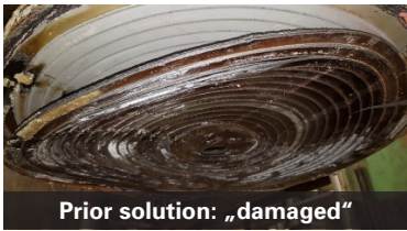
Lifting used GYLON EPIX® Style 3501-E EPX at disassembly.
